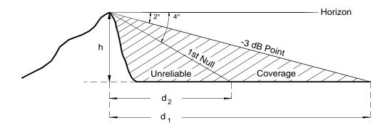
h = difference in height between the central station and the outstation antenna.
